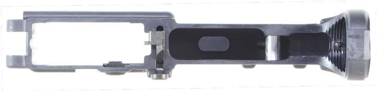
22. Both lower receiver walls thickened plus a bridge across the opening; the cavity is approximately 11 mm wide at the selector.
